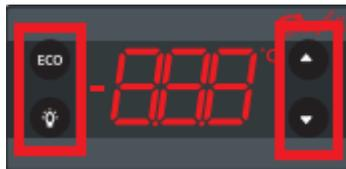
*Fig. 5. Control elements of the Danfoss controller ERC 112 .*
